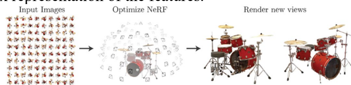
Figure 1 NeRF working block diagram. Using data from multiple perspectives for training, target locations in space have higher density and more accurate colors, prompting the neural network to predict a more continuous scene model.
